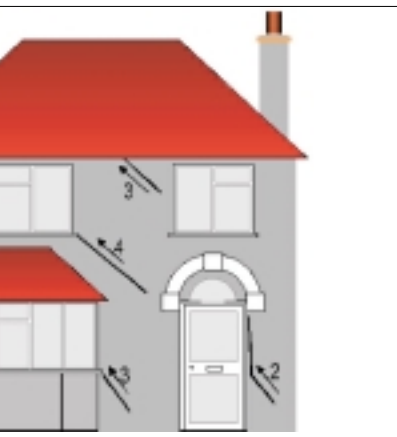
Fig 8. (above) Plot the cracks onto a drawing and note the crack widths in mm. The arrows indicate increase in widths of cracks
