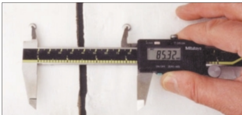
Fig 12. Monitoring with a digital caliper
