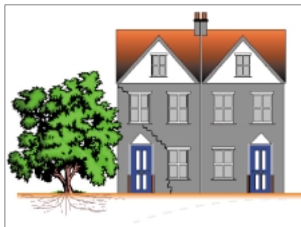
Fig 3. The foundation is subsiding due to action of the tree roots. The line of force is diagonal and the cracks are appearing perpendicular to the line of force. The cracks follow the line of weakness, in this case the window openings
