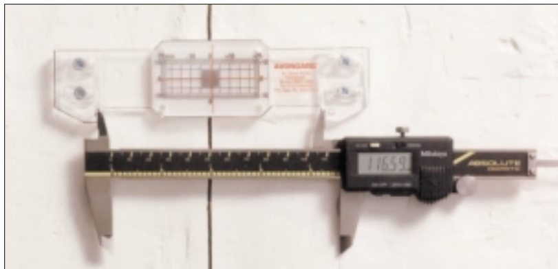
Fig 9. Use the type of gauge which has the facility to 'upgrade' the resolution of the readings to 0.1mm with precision calipers. This will give you the option to speed up the monitoring period if you are trying to identify trends of movement across the crack
